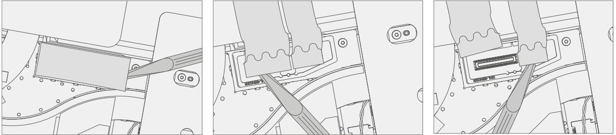
5. **Remove Residual IBC PSA** – Using flat side of a spudger, IPA, and cotton swabs, clean residual PSA off the IBC. Use only IPA and cotton swabs to clean the top edge. Ensure area around the Camera and IR Sensor is clean and free of any dust or other contamination. Wipe the area around the camera with a lint free cloth.
